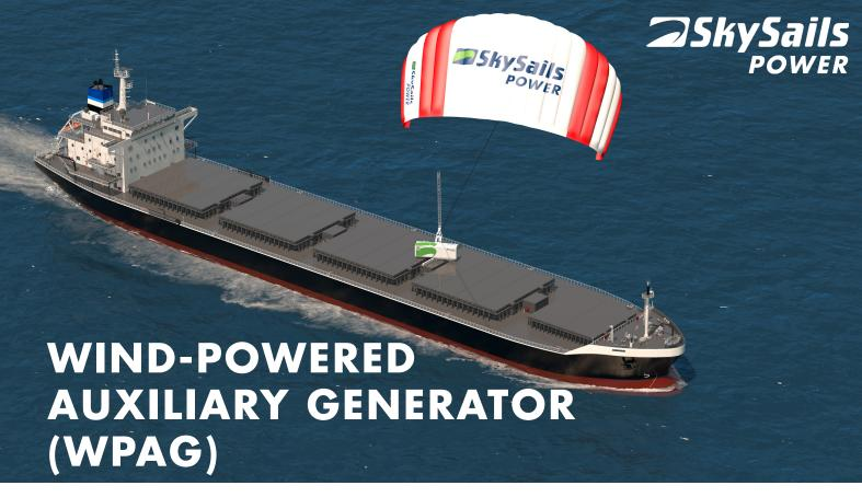
Auxiliary generators make up for 5 - 10%\* of the total fuel costs of a merchant vessel. The cost for generating onboard electricity with a Diesel-powered generator is very expensive and ranges from 12 to 16 US-\$-Cent per kWh at current fuel prices.
